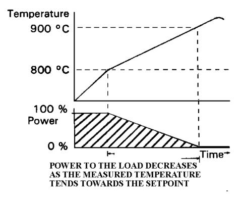
Proportional control in relay output controllers is normally achieved by varying the relay on/off time relationship. For example if the controller was calling for a 50% power output and the cycle time of the controller was 20 seconds the relay would be on for 10 seconds and off for 10 seconds. The cycle time of the Vertex on/off relay output controllers is approximately 15 seconds.
