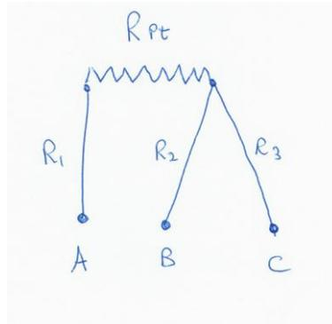
1. A PT100 normally has 3 wires. It is in simple terms a resistance that changes with temperature.
