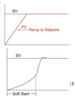
The "Soft Start" function allows you to limit the power applied to a load from initial startup ramping from 0% to 100% over the time you have set.
