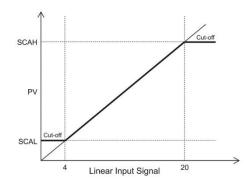
The Cut-off function is used to limit the input signal display (PV) within the limits defined by the user whenever the input signal is out of the scale defined by SERL and SERH. The cut-off function can be set to "Low", "High" or "High/Low" or set to "None" to disable it. The cut-off function has no effect for input signals other than linear types and is only showed when the input signal type is set to linear.
